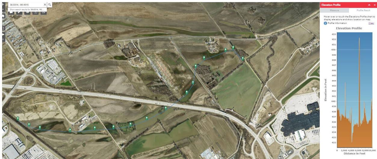
Figure 4 Elevation profile of Wetland A-B and its' relationship to the surrounding terrain.
